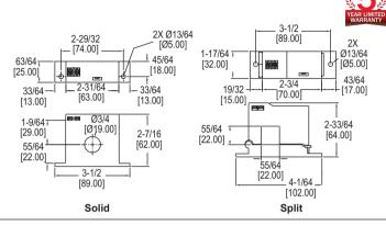
The Series CCT40/50 Current Transformers are a low cost alternative for measuring power and monitoring the operation of fans, pumps, or other equipment. For use on existing installations, split core models can be installed without disconnecting cables. Each model offers three jumper selectable ranges and a choice of three different outputs.
